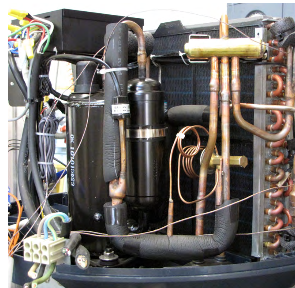
Interior components of a packaged heat pump.
